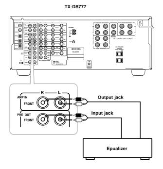
The AMP IN and the PREOUT FRONT connectors are attached with jumper plugs. When connecting an equalizer, remove these jumper plugs before connecting the audio connection cables.
